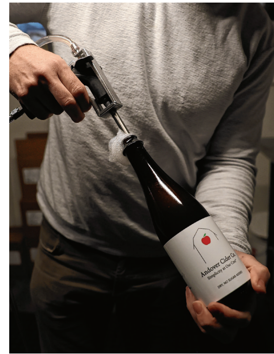
Caleb Harty uses a filling gun to transfer cider into a bottle.
