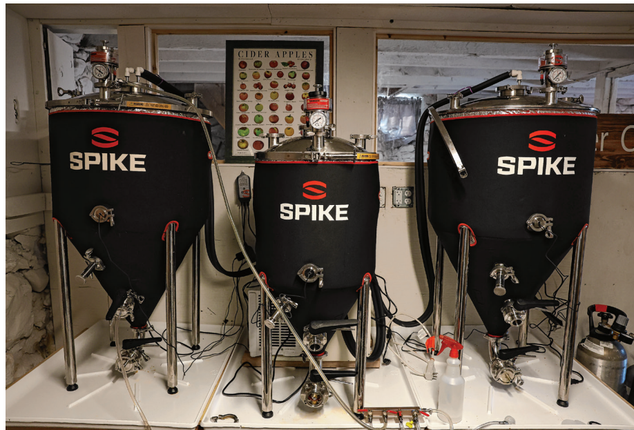
Stainless steel fermenters are temperature-controlled to aid in the cold crashing process, which allows yeast and other particles to settle at the bottom.
